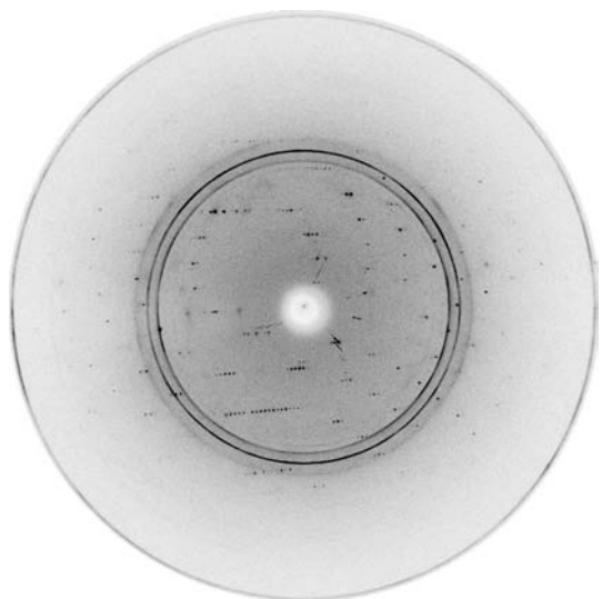
Figure 2 Diffraction image ( \Phi = 44.0 – 45.0^\circ ) of p73 \alpha residues 487–564. Note the presence of ice rings.
